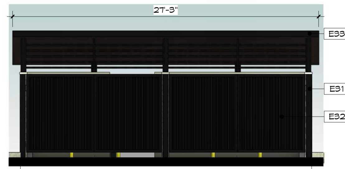
3 TRASH ENCLOSURE - NORTH ELEVATION 3/16" = 1'-0"
